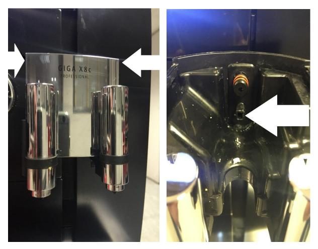
To remove the cover push the top two black tabs towards each other as indicated by the arrows in the left photo and slide upwards.
