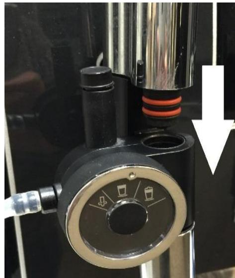
To remove the nozzle it needs to be unscrewed \***CLOCKWISE**\* as you look down from above, if the nozzle is stuck with dry milk you can use the pre-ground coffee spoon [located under the right flap on top of your machine] like a wrench to free it as in the picture
