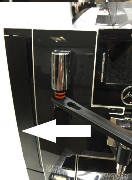
Once the steam nozzle has been removed, try the “1 portion milk button” if steam now comes from the machine you will need to clean out all the dry milk from the nozzle in the picture to the right.
