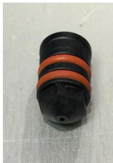
If the steam is coming correctly from the nozzle with the two red rings but no milk is being drawn through the milk frother there is probably a blockage.
